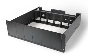
The Bluesound Professional RM160 is a rackmount system allowing up to 6 x B160S network streaming stereo amplifiers to be mounted in a 3U space in a 19" rack. The B160 modules slot in from the front and are secured by a front panel screw, allowing for swift replacement when required. B160S units are supported front and back and cabling is tidied with a rear tray.
